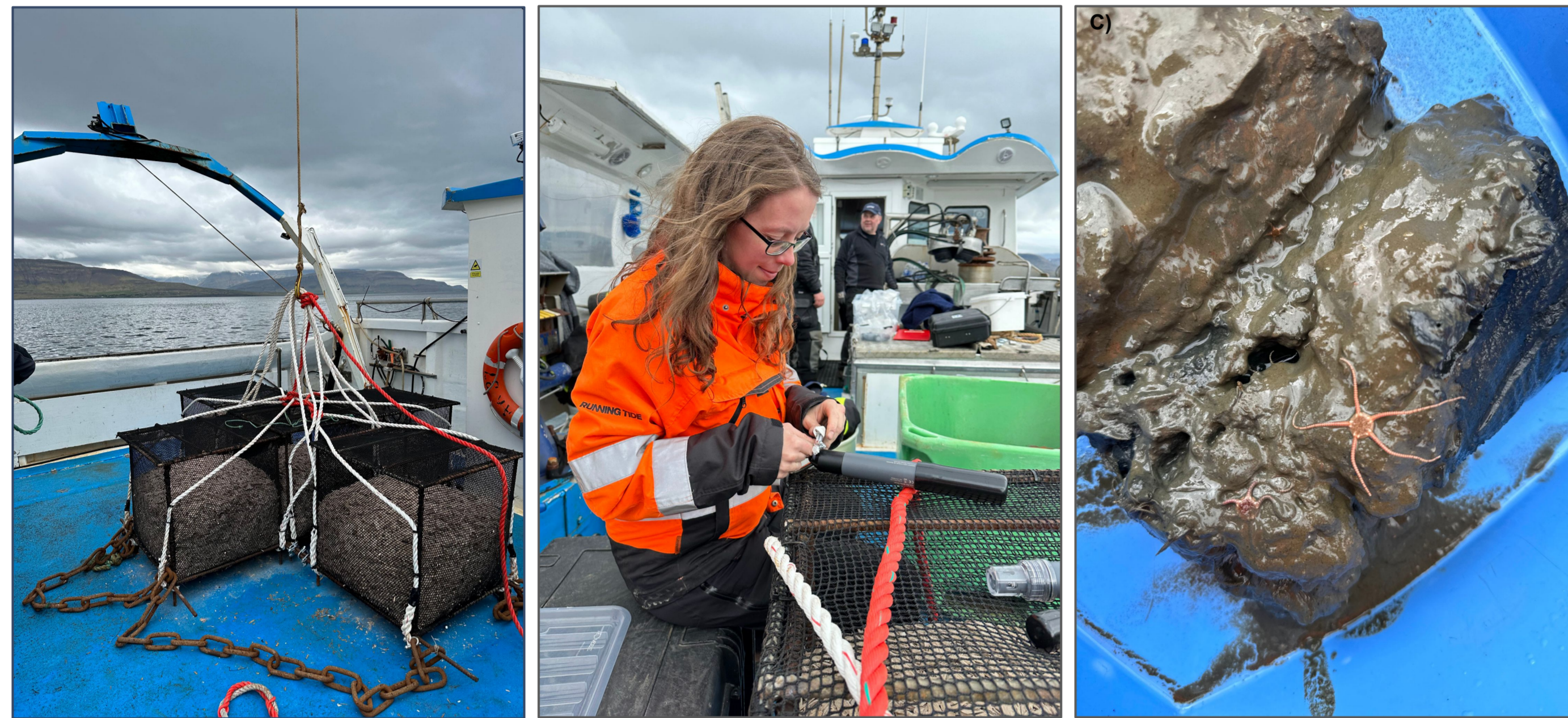
Figure 1. Setup of the Iceland Coastal Benthic Experiment (see below). From left to right: (A) The 5 experimental net cages next to the test site (30 m depth) in Hvalfjörður, Iceland. Each cage contains 100kg of wood coated with a mixture of CaCO 3 (80%) and Ca(OH) 2 (20%). (B) RT staff placing loggers to record dO, pH, temperature, and conductivity at test and control site. (C) Sediment at both sites was very fine grained (silt/clay) with detritus feeders such as brittle stars (Ophiuroidea) in abundance.
